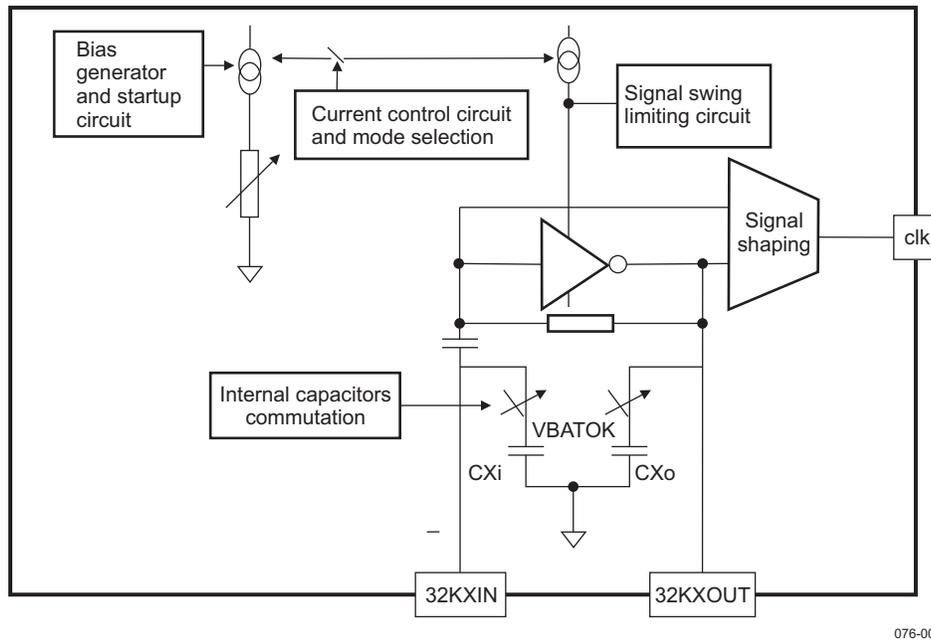
Figure 1. TPS659xx 32-kHz Internal Block Diagram
